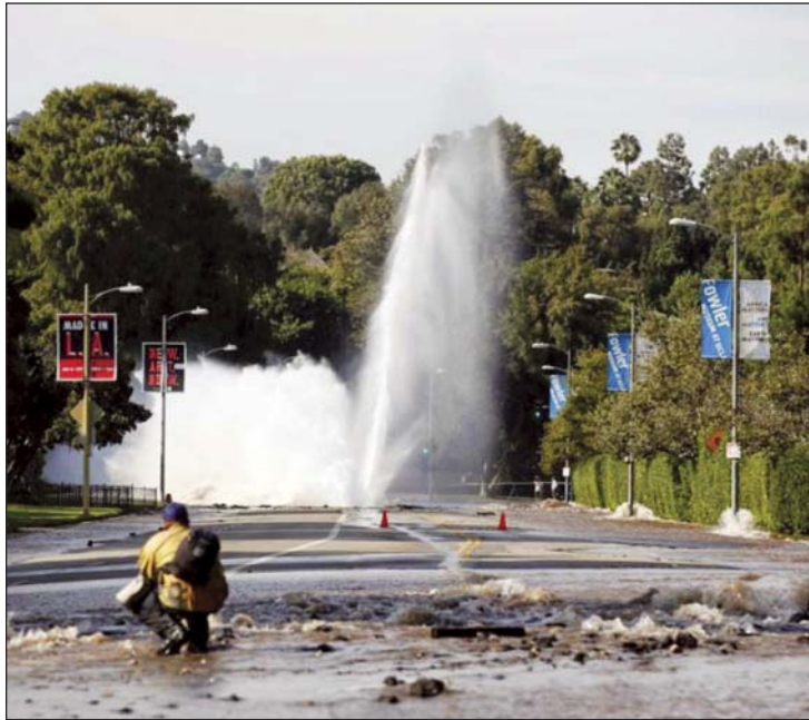
Figure 5. 30-in. Steel Pipe Failure at University of California at Los Angeles
